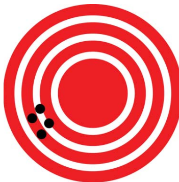
Figure 1.25 In this figure, the dots are concentrated rather closely to one another, indicating high precision, but they are rather far away from the actual location of the restaurant, indicating low accuracy. (credit: Dark Evil)
