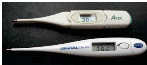
Figure 20.13 These familiar thermometers are based on the automated measurement of a thermistor's temperature-dependent resistance. (credit: Biol, Wikimedia Commons)
