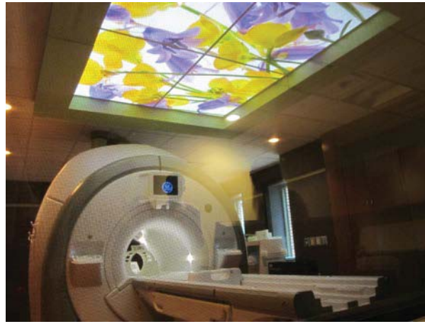
Figure 22.9 Instrument for magnetic resonance imaging (MRI). The device uses a superconducting cylindrical coil for the main magnetic field. The patient goes into this “tunnel” on the gurney. (credit: Bill McChesney, Flickr)
