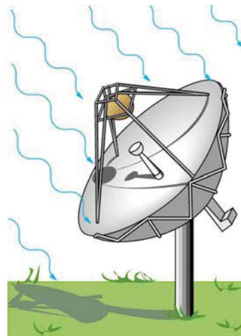
Figure 24.28 Satellite dishes receive TV signals sent from orbit. Although the signals are quite weak, the receiver can detect them by being tuned to resonate at their frequency.
