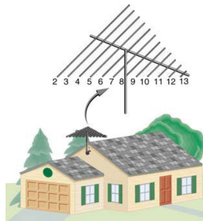
Figure 24.27 A television reception antenna has cross wires of various lengths to most efficiently receive different wavelengths.
