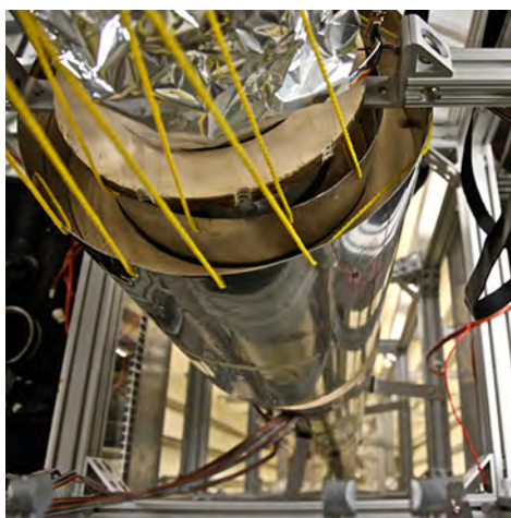
Figure 1.8 An atomic clock such as this one uses the vibrations of cesium atoms to keep time to a precision of better than a microsecond per year. The fundamental unit of time, the second, is based on such clocks. This image looks down from the top of an atomic fountain nearly 30 feet tall. (credit: Steve Jurvetson)
