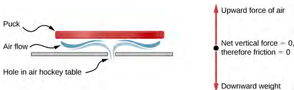
Figure 5.8 An air hockey table is useful in illustrating Newton's laws. When the air is off, friction quickly slows the puck; but when the air is on, it minimizes contact between the puck and the hockey table, and the puck glides far down the table.
