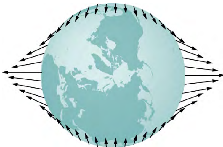
Figure 13.23 The tidal force is the difference between the gravitational force at the center and that elsewhere. In this figure, the tidal forces are shown at the ocean surface. These forces would diminish to zero as you approach Earth's center.
