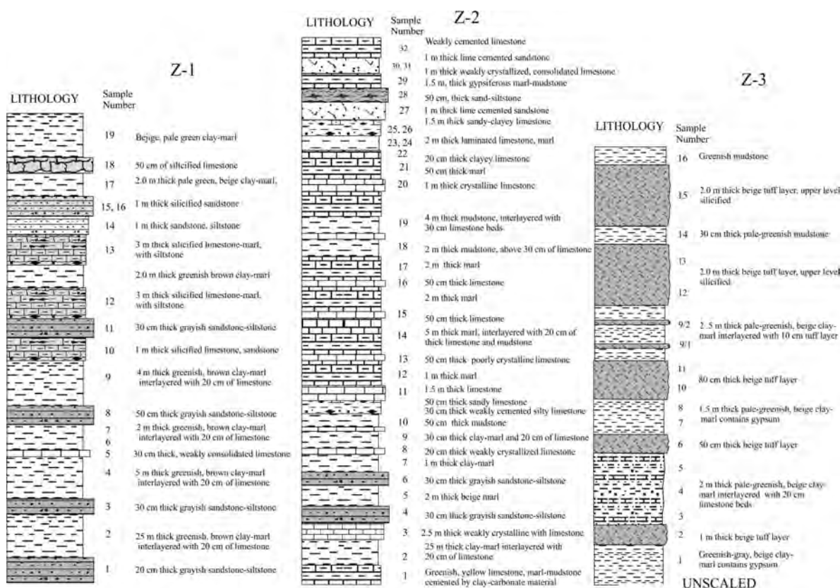
Figure 4. Generalized stratigraphic column of the Aktepe formation and Karacadağ volcano-sedimentary rocks. The figure also shows the detailed section of the stratigraphic interval sampled in the present study.
