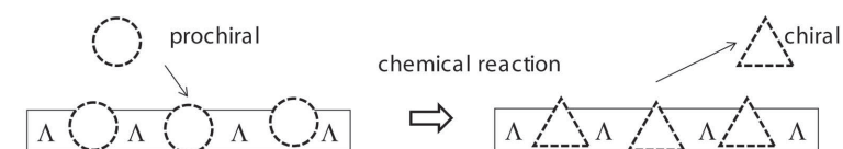
Figure 8. A schematic model for the transformation of a prochiral molecule to a chiral molecule under the steric control of chelates bound on a clay mineral surface.
