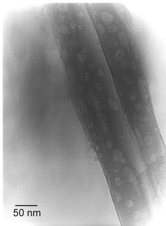
Figure 7. Halloysite crystal with core holes in a Ni-doped montmorillonite sample (43 \mu\text{mol/g} , 14 days' reaction time, sample A).
