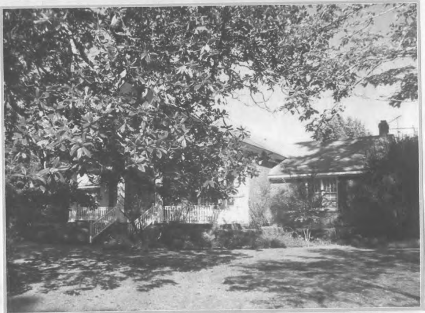
Groover – Boring – Winter – Jones...1851.....5207 Dixie Rd. Charlie Groover built this two story frame house made of hand hewn logs held together with wooden pegs. Dr. Thomas Boring bought the property in 1876 and it has remained in the family since that time. Now in 2013 it belongs to Dr. Baring's great, great, great, granddaughter Elizabeth Jones.
