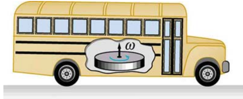
Figure 10.16 Experimental vehicles, such as this bus, have been constructed in which rotational kinetic energy is stored in a large flywheel. When the bus goes down a hill, its transmission converts its gravitational potential energy into \text{KE}_{\text{rot}} . It can also convert translational kinetic energy, when the bus stops, into \text{KE}_{\text{rot}} . The flywheel's energy can then be used to accelerate, to go up another hill, or to keep the bus from going against friction.
