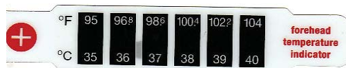
Figure 13.4 Each of the six squares on this plastic (liquid crystal) thermometer contains a film of a different heat-sensitive liquid crystal material. Below 95^{\circ}\text{F} , all six squares are black. When the plastic thermometer is exposed to temperature that increases to 95^{\circ}\text{F} , the first liquid crystal square changes color. When the temperature increases above 96.8^{\circ}\text{F} the second liquid crystal square also changes color, and so forth. (credit: Arkrishna, Wikimedia Commons)
