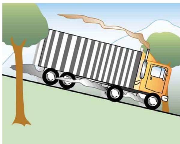
Figure 14.5 The smoking brakes on this truck are a visible evidence of the mechanical equivalent of heat.
