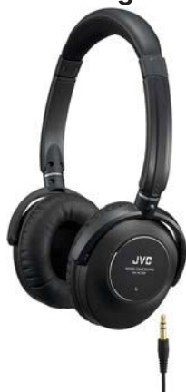
Figure 17.21 Some types of headphones use the phenomena of constructive and destructive interference to cancel out outside noises. (credit: JVC America, Flickr)
