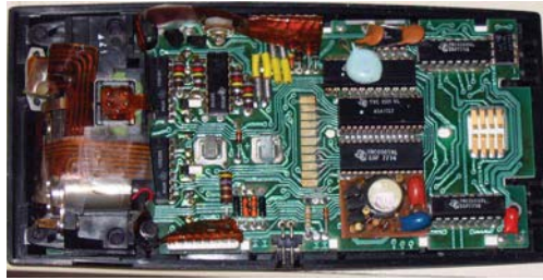
Figure 19.24 Energy stored in the large capacitor is used to preserve the memory of an electronic calculator when its batteries are charged. (credit: Kucharek, Wikimedia Commons)
