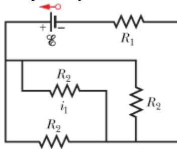
4. In the figure on the right, the ideal batteries have emfs  $\mathcal{E}_1 = 10.0 \text{ V}$  and  $\mathcal{E}_2 = 0.500 \mathcal{E}_1$ , and the resistances are each  $4.00 \Omega$ . What is the current in (a) resistance 2 and (b) resistance 3?
