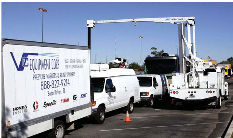
Figure 32.2 Customs officers inspect vehicles using neutron irradiation. Cars and trucks pass through portable x-ray machines that reveal their contents. (credit: Gerald L. Nino, CBP, U.S. Dept. of Homeland Security)
