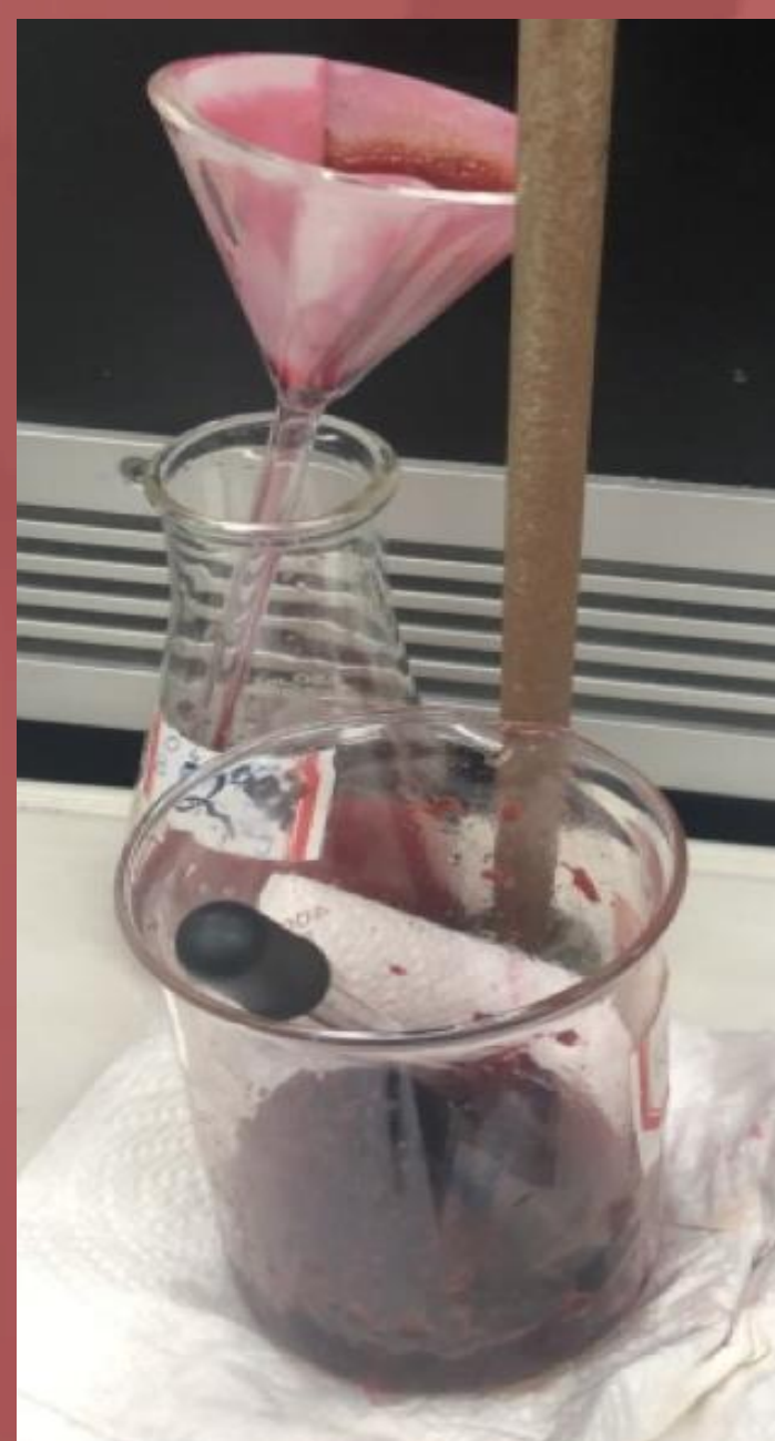
Figure 2. Cherry puree in large beaker. Funnel, filter paper, and filtrate in Erlenmeyer flask are behind.
