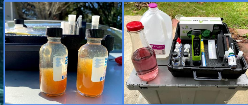
Dissolved Oxygen using the LaMotte shallow water testing kit
