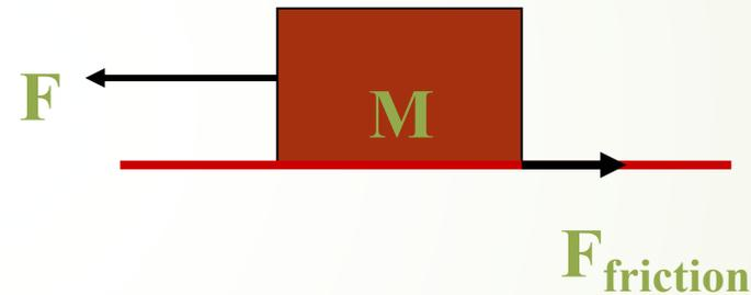
To Move M
