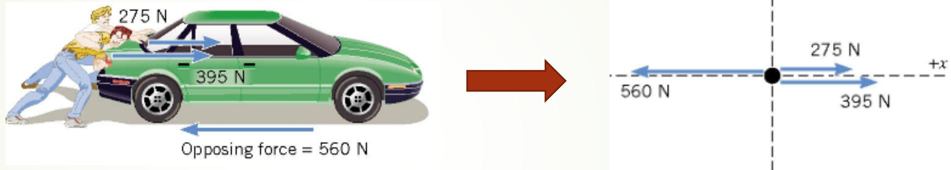
The net force in this case is:  $F_{net} = 275\text{ N} + 395\text{ N} - 560\text{ N} = +110\text{ N}$
