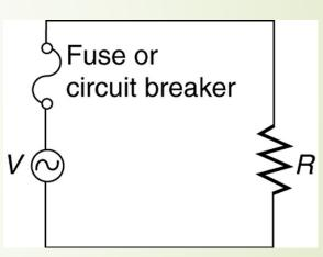
\*\*When a circuit carry more than a safe amount of current the circuit is said to be overloaded. When too many appliances are used at once in parallel combination, it may cause overloading of the circuit. We use fuses or circuit breakers to prevent damages to appliances and the circuit.
