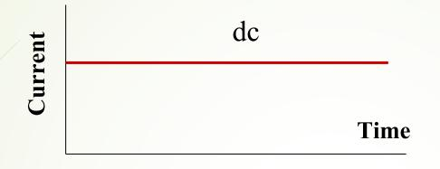
**Current flows in one Direction (e.g. Batteries)**
