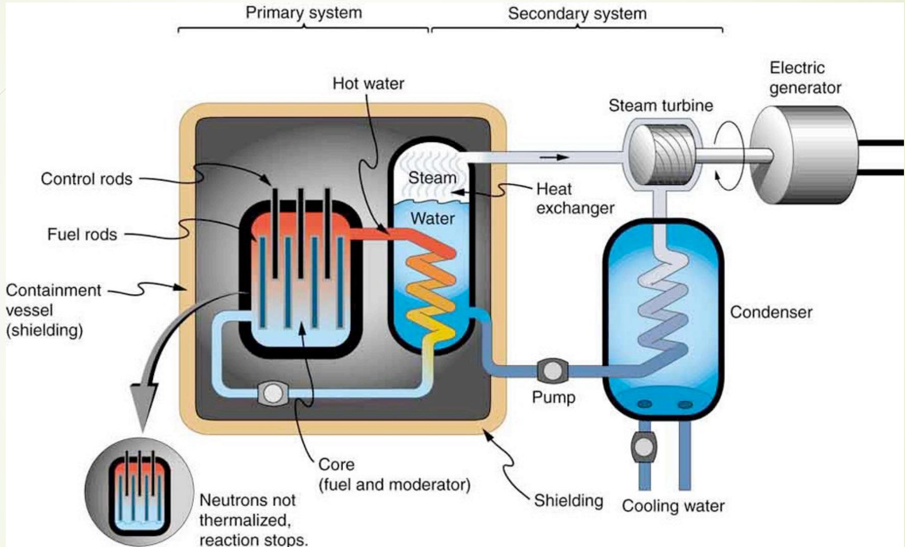
A pressurized water reactor is cleverly designed to control the fission of large amounts of  $^{235}\text{U}$ , while using the heat produced in the fission reaction to create steam for generating electrical energy.
