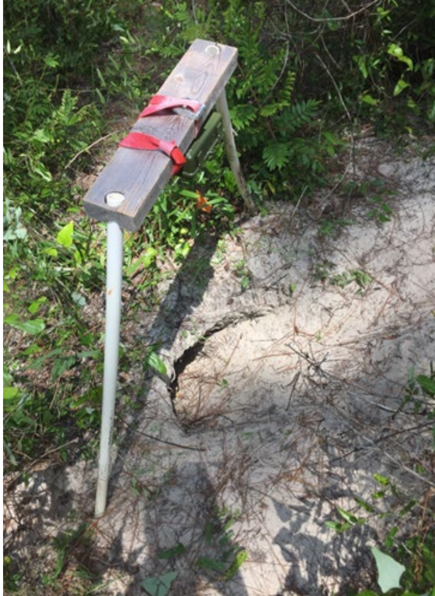
Figure 4. Example of camera trap setup at a gopher tortoise burrow. Camera mount legs are staked into the ground on either side of the burrow mouth as to minimize interference with burrow use by vertebrates. The camera lens is positioned to include the full burrow opening and only a small portion of surrounding ground on all sides of the burrow mouth in its field of view.
