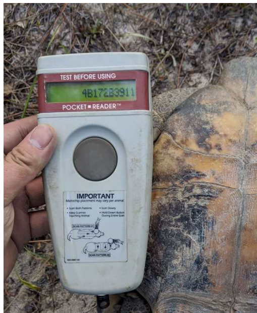
Figure 15: Handheld PIT tag Pocket Reader™ used to scan tortoises for PIT tags. PIT tags were scanned on the right anterior ventral leg.
