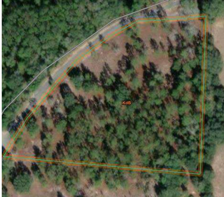
Figure 9: NRCS Web Soil Survey map of Pioneer Site (Pioneer) in Reed Bingham State Park, Cook County, Georgia, USA (Soil Survey Staff, 2020). Kershaw sand, 0 to 5 percent slopes (KdB) (orange acronym). Pioneer border (green line).
