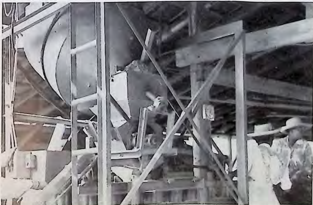
. . . the rotating soil mixer (upper left) and then on through the dispenser and into the cans. Employee whose hands are shown lower left is placing empty one gallon containers on the power driven conveyor belt. As the cans move down this belt, they are filled with a measured amount of potting or canning mix. A plunger packs them slightly and makes a hole for the potted liner, which is placed in the can by the employee at lower right. Other employees further on straighten and pack the plants before they leave the power driven conveyor to move by gravity conveyor to the wagons which in turn move them to their permanent location in the growing area. The plants are watered well before moving.
